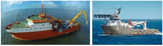
The cable lay vessel (approx. 90 POB) shall arrive at site fully laden with all equipment required to perform the installation activity. The method to transfer the plough from the vessel to the beach may require an additional abnormal load movement through Cork Port. However, it is envisaged that the plough shall be transferred on a shallow draft barge at high water and lifted by an on-board crane and placed in the receiving pit.
